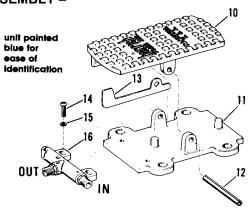
NO. 34-18 THREE-WAY HAND OPERATED VALVE ASSEMBLY –
